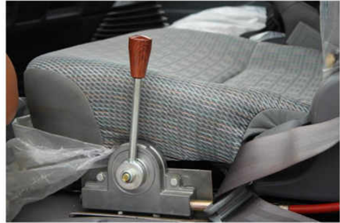
The Joystick at UPPER place The Man Lifter can work
